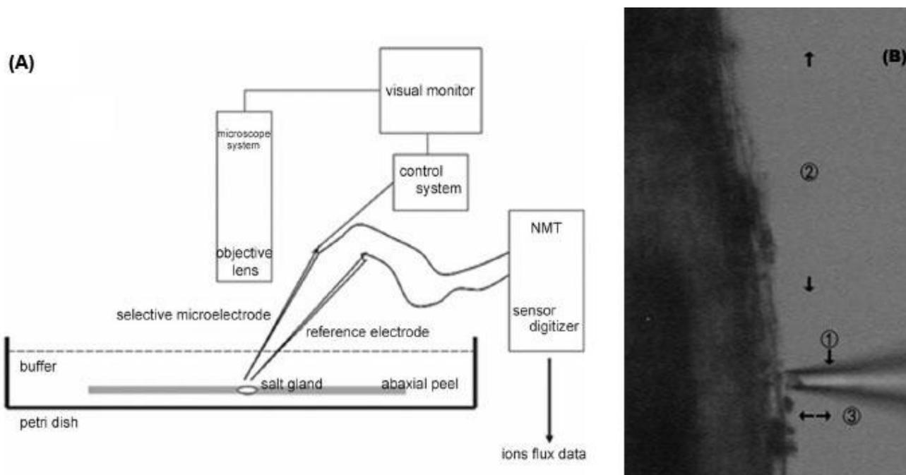
Fig. 3. Schematic diagram of NMT (non-invasive micro-test technology) system for measuring  $\text{Na}^+$  flux in roots of callus-cultured alfalfa lines exposed to seawater treatment. (A) The diagram showing the system used to measure selective ion flux from using a non-invasive ion-selective electrode. (B) A micrograph of electrodes (1) (locating at 500  $\mu\text{m}$  from the root apex (2)) movements between the two measuring positions (3) on the root surface.
