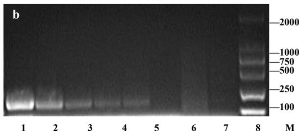
Fig. 4. The sensitivity detection of primers YF32/YR32 by real-time PCR amplification (a) and conventional PCR (b). (a) 1-6, 1ng/μL, 100pg/μL, 10pg/μL, 1pg/μL, 100fg/μL, 10fg/μL Psa genomic DNA; 7, ddH<sub>2</sub>O. (b) 1-7, 10ng/μL, 1ng/μL, 100pg/μL, 10pg/μL, 1pg/μL, 100fg/μL, 10fg/μL Psa genomic DNA; 8, ddH<sub>2</sub>O; M, DL2000.
