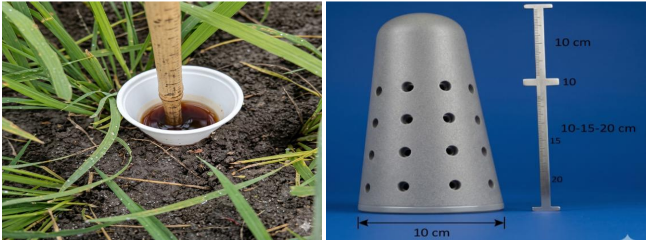
Fig. 1. Field Perforated tube technique for tracking the recession of water levels to depths of 10, 15, and 20 cm as a signal for irrigation replenishment.
