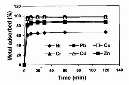
Figure 1. Biosorption of heavy metals by *Phormodium* biomass as a function of time.
