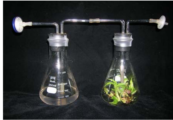
Fig. 1. The modified TIS apparatus used in the experiments.
