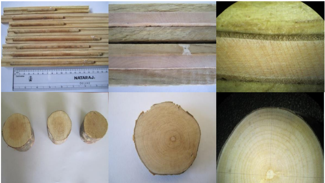
Fig. 7. Tree cores and cut stumps samples and after sanding with 1000 grits of sandpaper.
